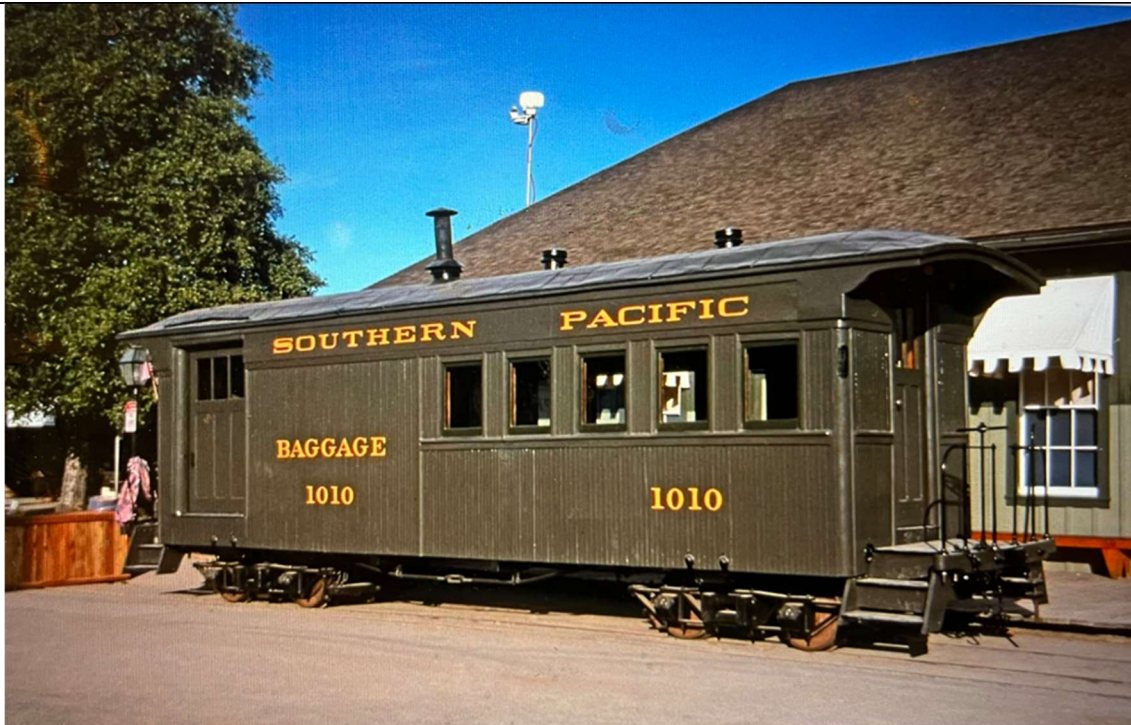
SOUTHERN PACIFIC COMBINE # 1010 - Car 1010 was built by the San Joaquin & Sierra Nevada Railroad in their shops near Lodi, California in 1882. The car's original number is not currently known. Originally built as a coach, the car was later converted to a combine. The SJ&SN was sold to the Southern Pacific in 1885. The SP merged the SJ&SN into its Northern Railway subsidiary where the car was numbered 1010. In 1904 the SP standard gauged the line and the car was transferred to the SPC, where it was used until 1907. It was then sent to the N&C where it became car 16. In late 1913 the car was set aside at Mina, Nevada and converted to a house for railroad workers. It was purchased by Richard Datin in 1960. He sold it to SPCRR in 1990. (Don Marenzi collection)
