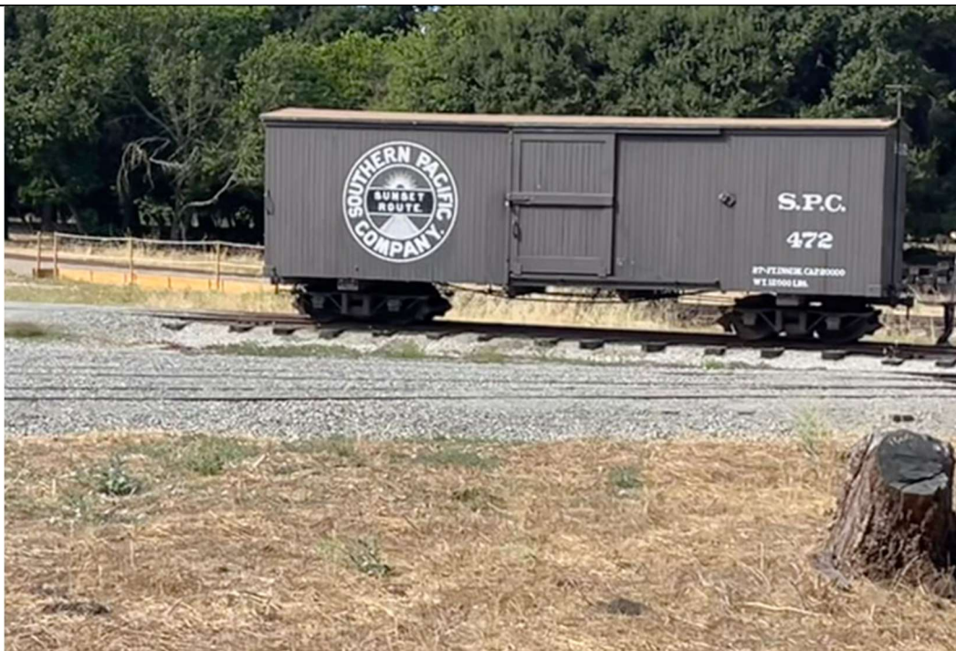
BOXCAR #472 - South Pacific Coast (subsidiary of Southern Pacific Company) boxcar #472 was originally built for the Oregonian Railway. It is a typical Carter Brothers car. It was transferred to the Southern Pacific-owned South Pacific Coast after 1887. When the SPC was standard gauged in 1906, it was transferred to the Nevada & California subsidiary of the Southern Pacific RR.
